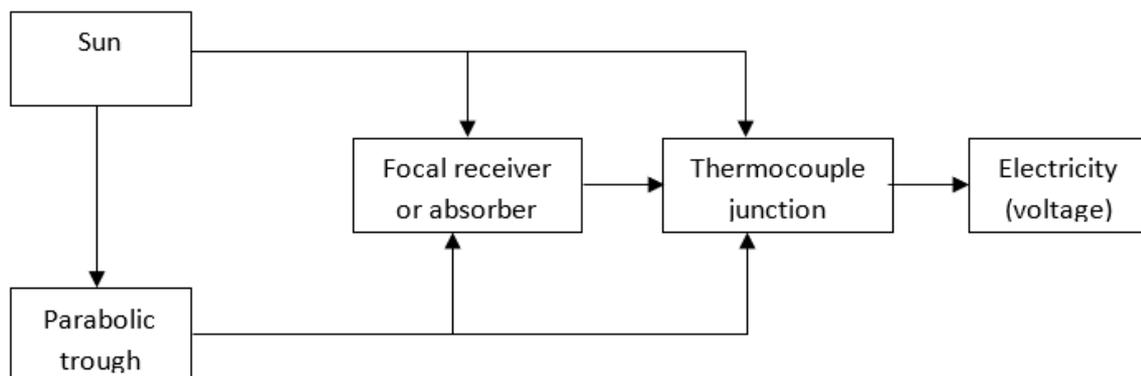
Figure 1: Block diagram of solar thermal electricity generation
